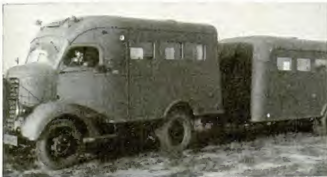
Above, interior view of the "broadcasting station on wheels" (below) used by the Signal Corps. Trailer carries radio receiver, also motors to supply power for a transmitter in the tractor
